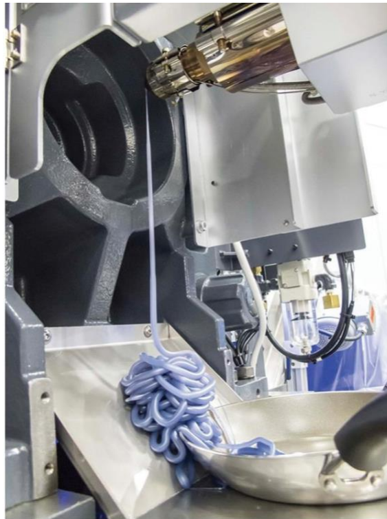
Figure 6 - Typical Purge & Guarding
