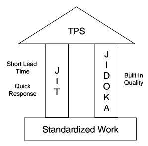
It is a pictorial representation of the principles and strengths of the Toyota Production System (TPS). The foundation of TPS is standardized work. The two major pillars supporting TPS are just-in-time (JIT) and jidoka, (also known as autonomation) or as I call it, stop the line, fix the problem.
