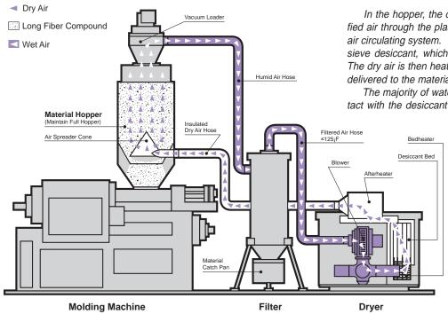
In the hopper, the drying units force hot dehumidified air through the plastic granule by way of a closed air circulating system. The moisture is removed by the sieve desiccant, which traps the moisture molecules. The dry air is then heated to a preset temperature and delivered to the material in the insulated hopper.
