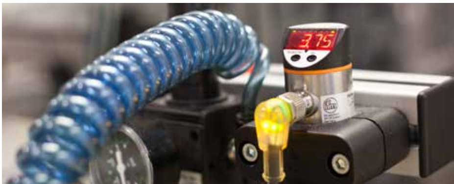
Figure 12: Digital display of a defined process parameter. The process parameter may only be adapted by an authorized associate with a key.
