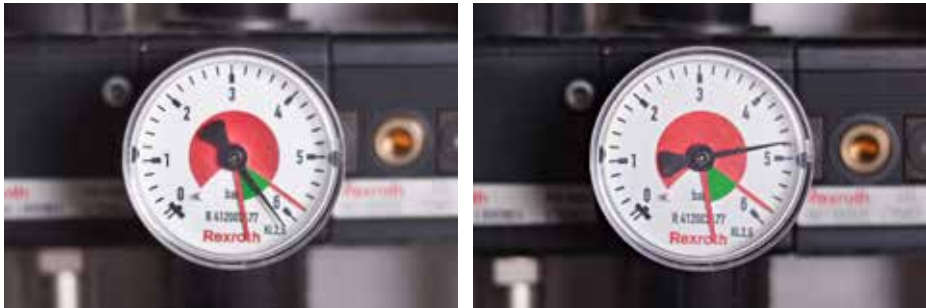
Figure 11: Color coding of tolerance range; left: tolerance adhered to, right: process parameter outside tolerance range
