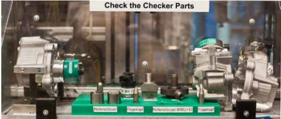
Figure 18: "Check the checker" parts (test dummies)
