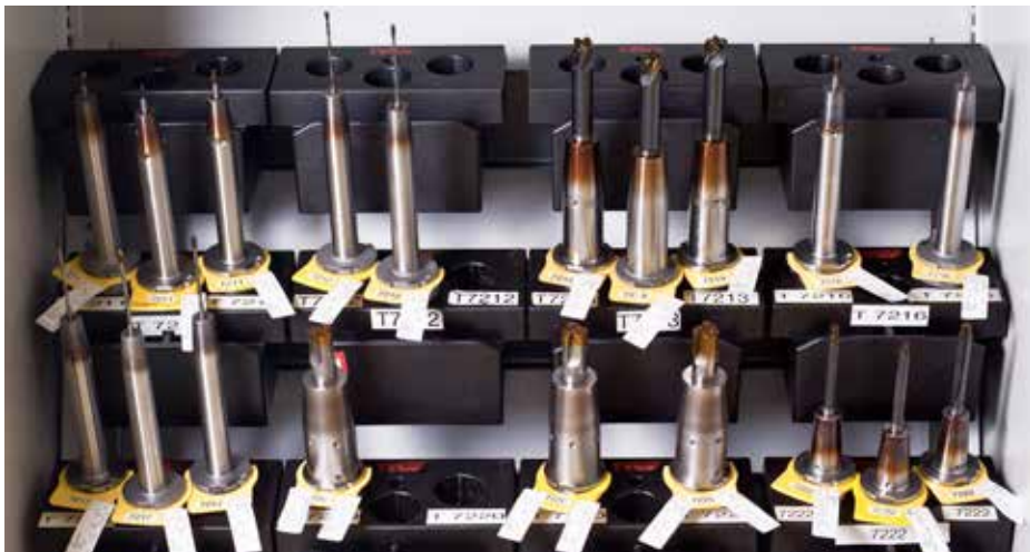
Figure 24: Storage of wear-prone tools including state description and service life specification
