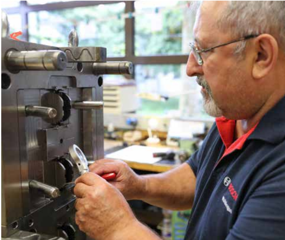
Figure 21: Checking of a complex tool for damage and wear by an expert
