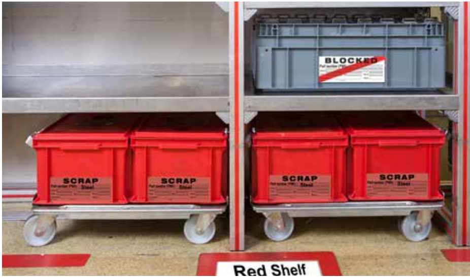
Figure 30: Red shelf with scrap and blocked goods
