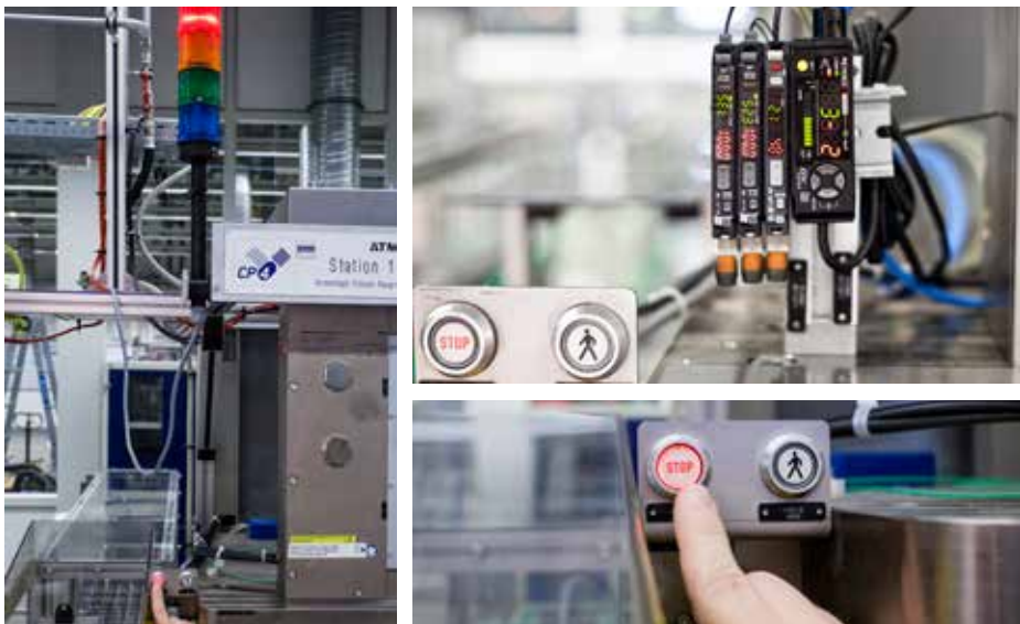
Figure 4: Implementation examples of the “Andon Cord” principle with a stop button
