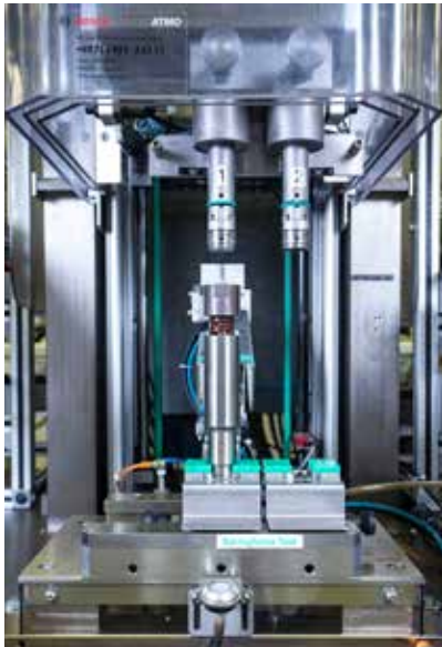
Figure 16 (left) and Figure 17 (right): Application of "check the checker" through inspection of the insertion force sensor using a spring force dummy
