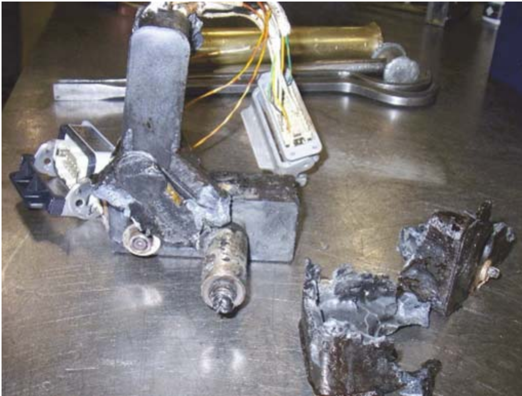
Figure 1.4 Effect of jumping to action without understanding the problem: a hot runner manifold encased in plastic
