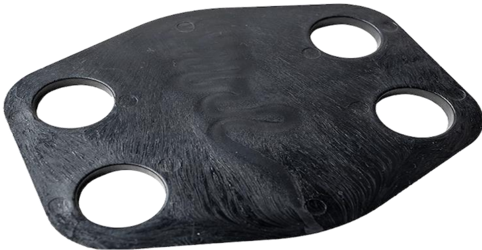
Figure 10 - Jetting in a Molded Part
